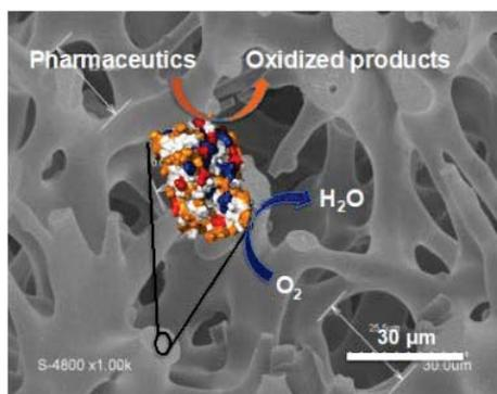
**Figure 1:** SEM image of the macropore structure of silica monoliths and schematic representation of laccase immobilized in the mesopores with an illustration of the oxidation mechanism of micropollutants.
